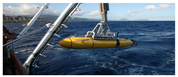
The fully air transportable Echo Mapper Autonomous Underwater Vehicle (AUV) is one of the multiple AUV solutions offered by Fugro worldwide. Echo Mapper is a Bluefin 21 AUV and is operated by Fugro Seafloor Surveys, Inc., in Seattle.
